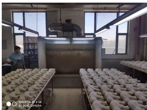
喷漆房-废气收集措施-水帘柜
